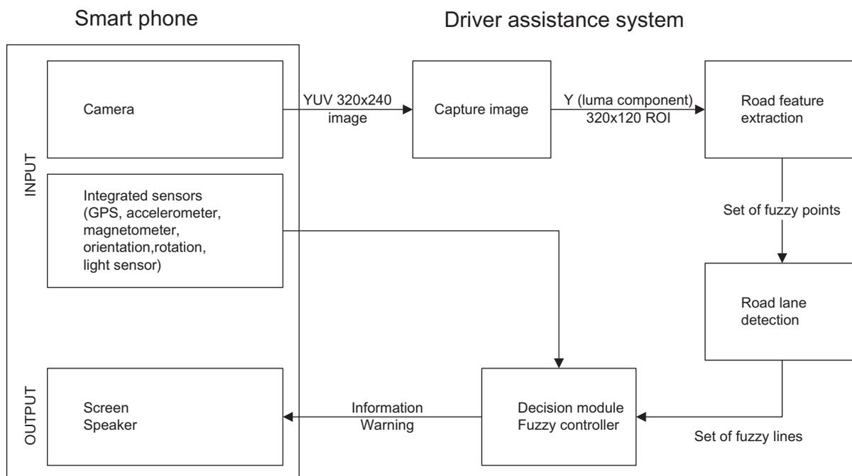
Fig. 2.1. Conceptual schematic of a driver assistance system integrated into a smart phone.
