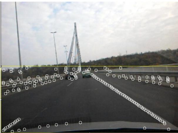
Fig. 2.3. Extracted set of fuzzy points. Each fuzzy point is represented as a white circle.
