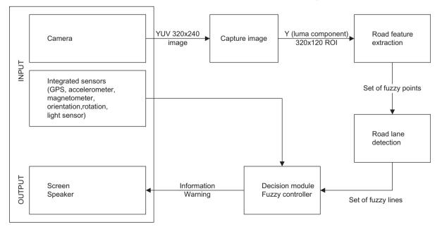
Fig. 2.1. Conceptual schematic of a driver assistance system integrated into a smart phone.
