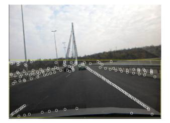
Fig. 2.3. Extracted set of fuzzy points. Each fuzzy point is represented as a white circle.
