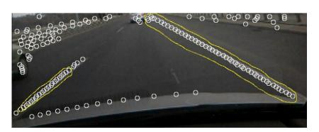
Fig. 4.1. Example of two initial "line like" fuzzy connected sets of fuzzy points.
