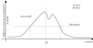
Fig. 3.2. Imprecision in edge detection.
